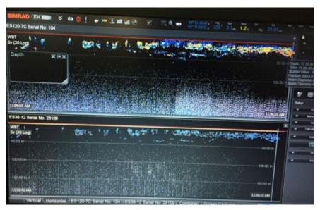
**Figure 8.** Acoustics trace of large, shallow (top 25m) krill school detected during acoustics survey in Process Study 1. Data from the EK80 echosounder mounted on acoustics towfish; upper panel is 120 Khz, lower is 38 KHz frequency.
