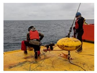
**Figure 2.** Recovery of the 300.100 mooring, with the top float sitting on the back deck. MT Josh Mitchell and MLT Diane Hutt were instrumental in a smooth and successful recovery.
